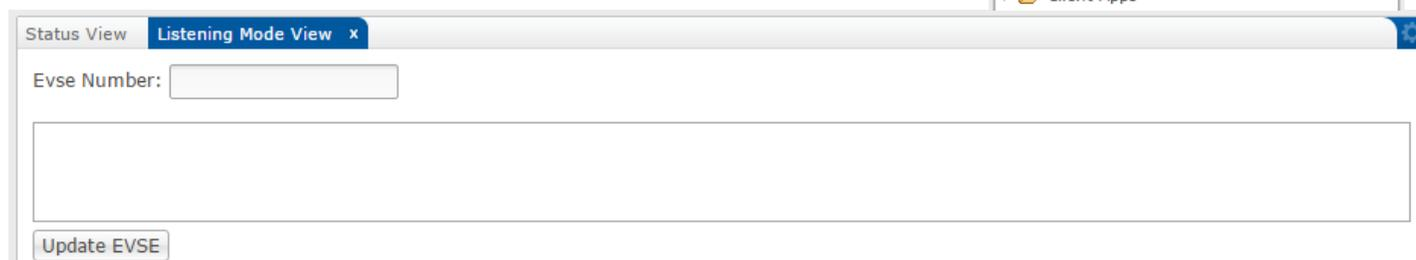
5. The Gateway Module is now in Listening Mode and will find the EVSE. The EVSE's ZigBee Module ID will display in the empty area of the screen. This might take a minute or two.
